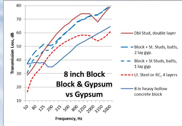
weaker at many frequencies but better at low frequencies. However, notice that with the gypsum added, the block wall can be weakened at low frequencies.
