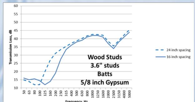
frequencies, there is a structural resonance related to the overall stiffness of the assembly. When the studs are very stiff as wood and closely spaced, this resonance increases to a higher frequency above 125 Hz and significantly reduces the performance at 125 Hz. In the chart on Page 2 this structural resonance has been introduced for both the 24 and 16 inch spacing to illustrate the effect.
